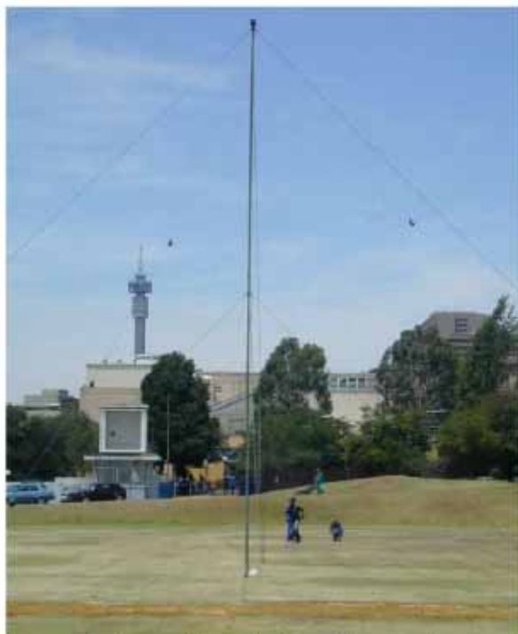
Antenna Mounted on 10m mast
